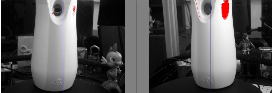
An example of strong external lighting - the backlight is not contrasting.
