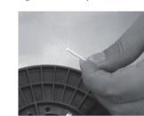
Insert the filament into the tube until it comes out from the other end of the tube. The tube with the filament cross the hole of the printer top door.
